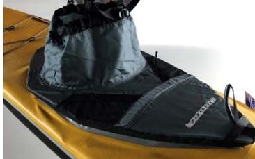
Skirt Installed over spray deck.
